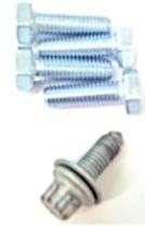
1. Start by positioning the car on flat level ground. Pop the hood and remove the 2 front and 2 inner bolts on each strut tower. They may be either 13mm head or #12 External Torx depending on year and updates to the car.
