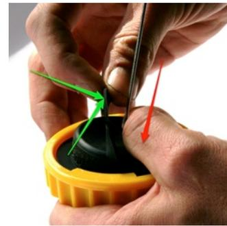
4. Now that the dipstick assembly is all apart, reverse the disassembly to install the new cap. Start with the cap upside down. Place the spring around the flange built into the new cap. Place the black plastic and dipstick piece on top of the spring.
