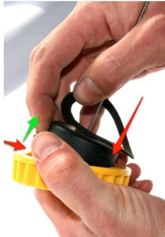
3. Once the seal ring is out, press down on the black plastic below one of the keeper tabs (Large red arrow to left) and rock the assembly out by pulling up on the other side of the black plastic (Green arrow to left). It may take a bit of force to get it past a keeper tab on the old cap, but it should come out pretty clean. Be careful to watch for the spring as it is between the black plastic and the old cap.
