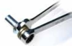
•While tightening the bolt you will feel a spike in the required torque and then as the rivet deforms you will be able to feel it bottom indicating it is done. To double check you can attempt to spin the assembly with the nut /wrench. It should be pretty tight if not tighten the bolt a bit more.
