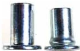
This shows the before and after of the rivet installation. In actual use the subframe would be between the bulge and the washer head of the rivet. Once installed in a blind hole the rivet grabs onto the metal inside the hole. This is not as hard as it sounds, Really!
