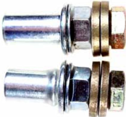
•First, assemble the tool as shown in the images to the left. The rivet will slide into the subframe hole. A dab of grease on the threads and on the washers will help but is not necessary.
