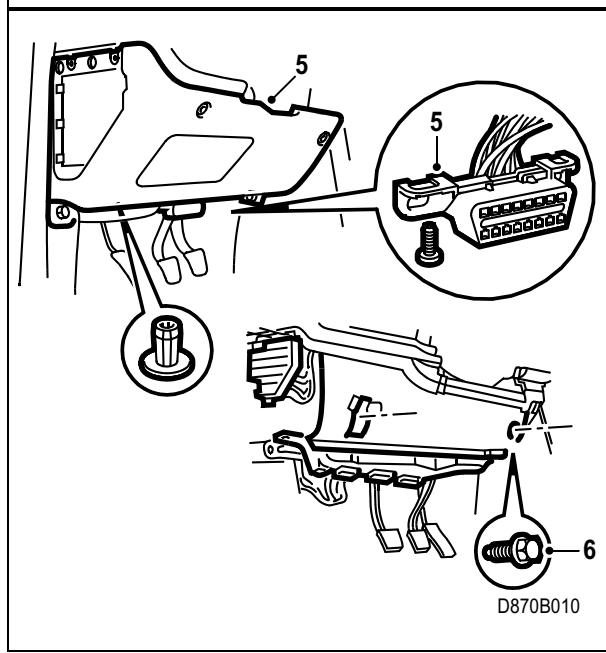
7 Loosen the screws and move the fuse board aside.
