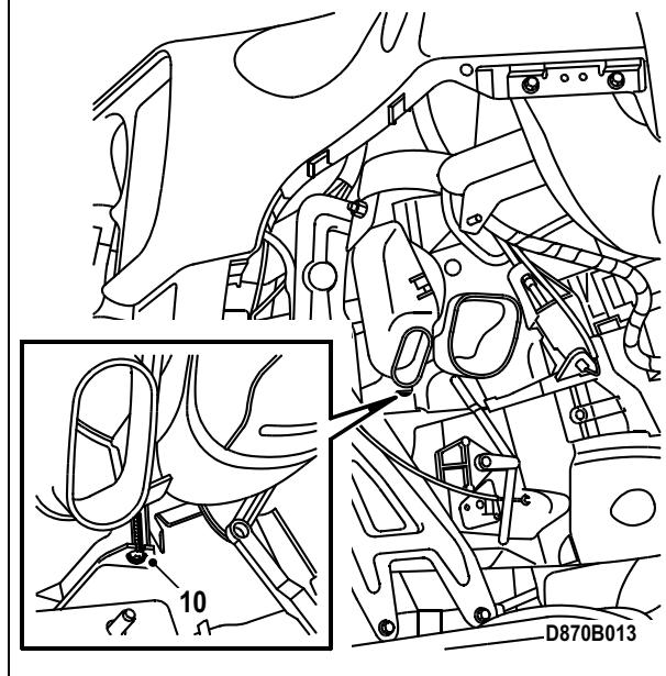
11 Remove the screw on the left-hand side.
