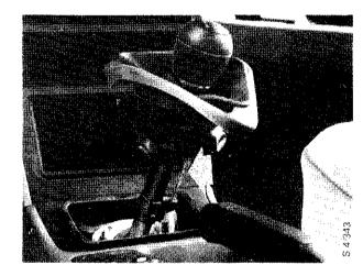
2 Connect the selector rod to the selector-rod universal joint and tighten the pinch-bolt.
